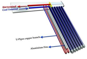
There are many types of vacuum tubes which are used in a number of fields for heating water. Double glass pipes are the most common in use.
